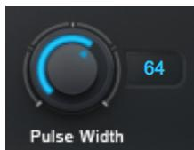
The **Glottal Pulse Width** control lets you select the pulse width of the modeled glottal waveform.
