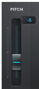
The **Pitch** control lets you shift the pitch of the input voice up or down by semitones. The range is from -12 (one octave down) to 12 (one octave up).
