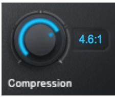
The **Compression** control sets the ratio of the compressor, which determines how much gain reduction is applied when the sibilant signal exceeds the threshold. Higher compression ratios result in more gain reduction.
