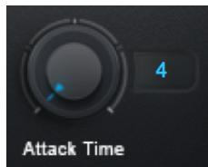
The **Attack Time** control determines how quickly gain reduction is applied when the sibilant signal exceeds the threshold.
