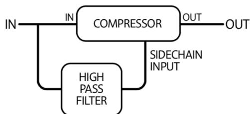
A high pass filter is used to isolate the sibilant sounds from the rest of the vocal track.
