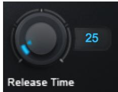
This **Release Time** control sets the time it takes the compressor's gain to increase 6 dB after the sibilant signal drops below the threshold.
