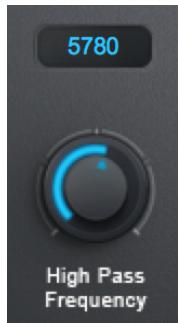
The **High Pass Frequency** control sets the frequency of the high pass filter, which is used as a sidechain input to the compressor.
