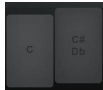
When a note on the Keyboard is set to Off, it will appear grey, and any incoming pitches that are closest to that note will be tuned to the next closest scale note instead.
