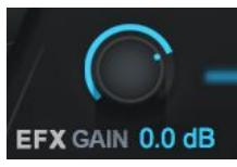
The EFX Gain knob controls the level of the audio at the input of the Auto-EFX multi-effects rack (after Auto-Tune processing). Use it, in combination with [EFX Output Meter](#), to regulate gain and avoid clipping.
