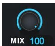
The Mix control allows you to mix in the “dry” unprocessed audio of your track with the processed output Auto-Tune EFX+. When mix is set to 100%, only the processed signal is present in the output.
