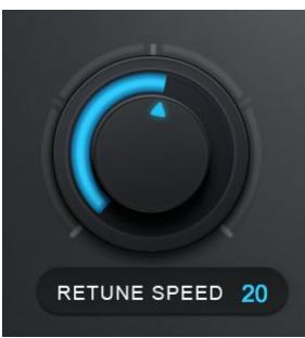
Retune Speed controls how rapidly the pitch correction is applied to the incoming audio. A zero setting will cause immediate changes from one pitch to another, and will completely suppress any vibrato or deviations in pitch.
